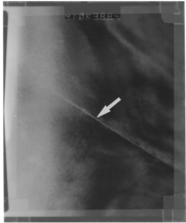
Figure 6 Transmission electron micrograph (bright-field image) of BMT-0.02WO 3 sintered at 1600°C for 4 hrs ( \times 410,000 ).
